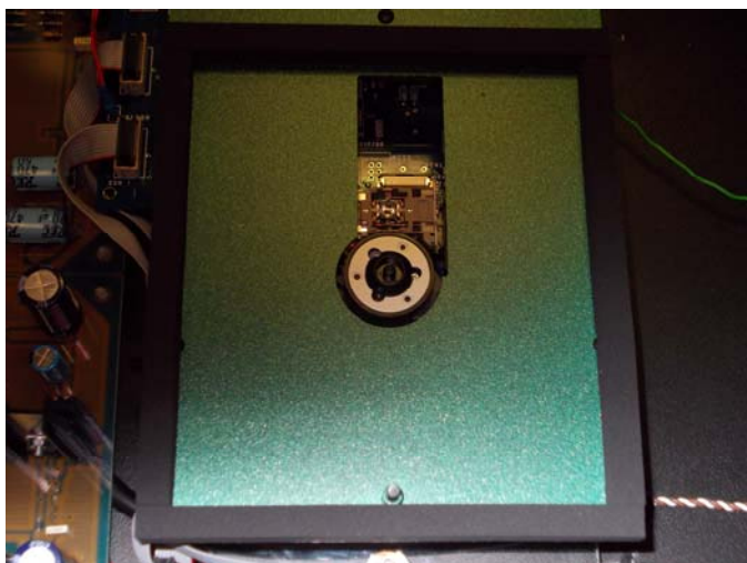
Alluminium cover with green painting Rubber foam frame
